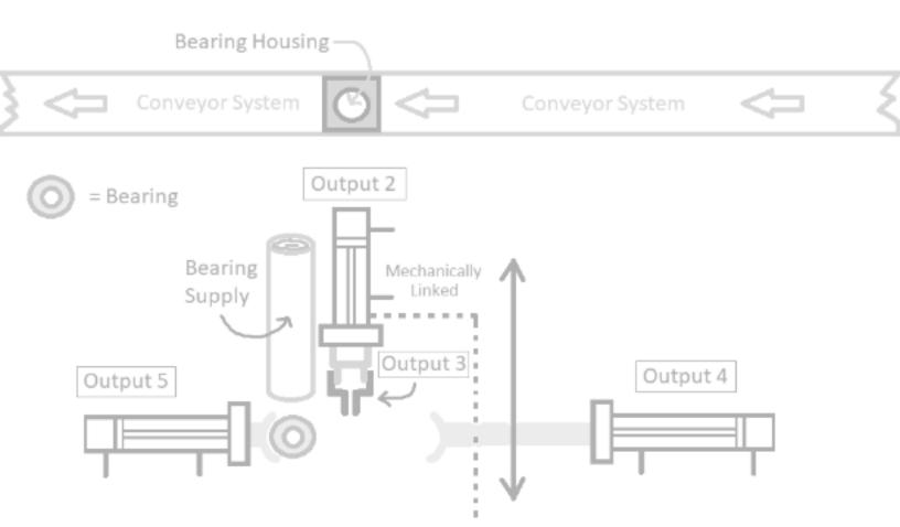
Bearing Supply, Sorting, & Placement Automated System
