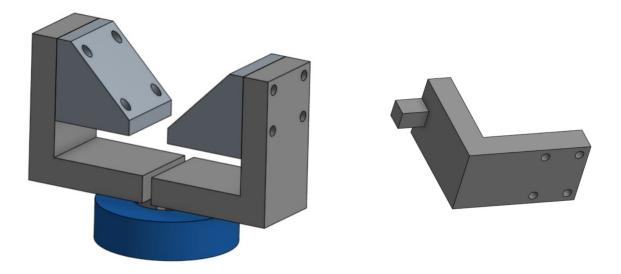
The blue cylinder is the bearing and the grey parts are what I designed. The triangle shapes show what part I had to attach to.
